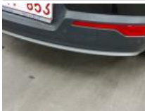
Bumper R, Dent(s) and scratch(es), Spot repair
