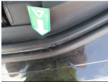
Door entry seal / Back / Broken
